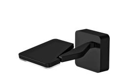
Wall lighting fixture for interiors, with swivelling light beam. Pickled sheet metal wall bracket in polyacrylic paint. Die-cast aluminium wall plate in polyacrylic paint. Die-cast aluminium structure in white, black, red or titanium polyacrylic paint. Die-cast aluminium head rotating on two axes in polyacrylic paint. Modelled acrylic diffuser with mat finish and double serigraphy. Push-button to adjust luminosity according to 5 levels of visual comfort.
