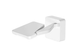
Wall lighting fixture for interiors, with swivelling light beam. Pickled sheet metal wall bracket in polyacrylic paint. Die-cast aluminium wall plate in polyacrylic paint. Die-cast aluminium structure in white, black, red or titanium polyacrylic paint. Die-cast aluminium head rotating on two axes in polyacrylic paint. Modelled acrylic diffuser with mat finish and double serigraphy. Push-button to adjust luminosity according to 5 levels of visual comfort.
