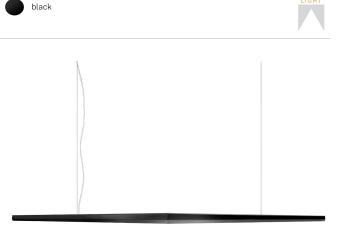
Suspension lighting fixture for interiors, with direct light emission. Machined aluminium structure in white or black polyacrylic paint. Anodized extruded aluminium heat sink. Extruded polycarbonate diffuser with opaline finish. Suspension kit with griplocks and 2m (78,7") long steel cables. 2,3m (90,6") long power cable in transparent PVC. Power canopy with galvanized sheet metal ceiling bracket and pickled sheet metal covering in white or black polyacrylic paint.
