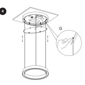
**G:** To adjust the cable height, push the metal cable adjuster and either pull or feed the cable to the desired length. Release the cable adjuster to secure the cable.
