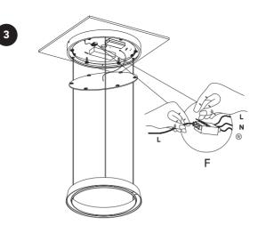
F: Connect the cables from both the lamp and the mains power into the terminal as illustrated above.
