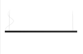
Suspension lighting fixture for interiors, with direct light emission. Extruded aluminium structure in RAL 9003 white powder paint. Extruded aluminium reflector in powder paint. Extruded polycarbonate diffuser with opaline finish. Aluminium end caps in polyacrylic paint. Suspension kit with griplocks and 2m (78,7") long steel cables. 2,2m (86,6") long power cable in transparent PVC. Power canopy with pickled sheet metal ceiling bracket and covering in white polyacrylic paint.
