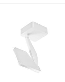
Ceiling or wall lighting fixture for interiors, with swivelling light beam. Pickled sheet metal ceiling/wall bracket in polyacrylic paint. Die-cast aluminium wall plate in polyacrylic paint. Die-cast aluminium structure in white, black, red or titanium polyacrylic paint. Die-cast aluminium head rotating on two axes in polyacrylic paint. Modelled acrylic diffuser with mat finish and double serigraphy.
