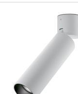
Ceiling or wall lighting fixture for interiors, with swivelling light beam. Ceiling/wall plate in die-cast aluminium with polyacrylic paint. Electrical connection housing in die-cast aluminium with polyacrylic paint. Die-cast aluminium joint with polyacrylic paint. Die-cast aluminium structure rotating on two axes in white, black, bronze, mat brass or titanium polyacrylic paint.
