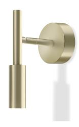
Ceiling or wall lighting fixture for interiors, with swivelling light beam. Galvanized sheet metal ceiling or wall bracket. Die-cast aluminium wall plate in white, champagne, mat black, bronze or titanium polyacrylic paint. Turned brass joints in polyacrylic paint. Turned aluminium structure in polyacrylic paint. Turned aluminium head rotating on two axes in polyacrylic paint. Modelled polycarbonate diffuser with opaline finish.
